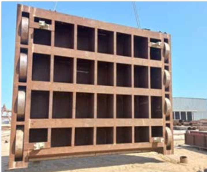
Working lock - 47 tons
